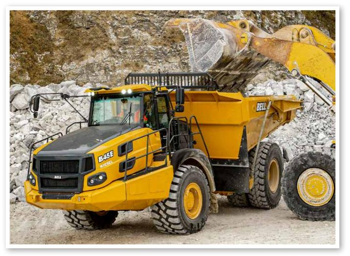
The exhaust gas-heated 25m<sup>3</sup> bin with a standard width of 4 265 mm (with tailgate: 26m<sup>3</sup>/4 639 mm) also marks the vehicle width, however, a narrower "Narrow" bin option of the same volume, brings the width of the Bell B45E 4x4 to less than 4m.
