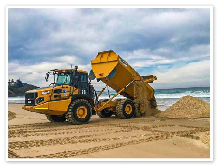
The ADT fleet is used mainly by the civil construction industry for bulk earthworks and trucks are generally replaced between 10 000 and 15 000 hours to ensure the mechanical availability of the fleet is kept high.
