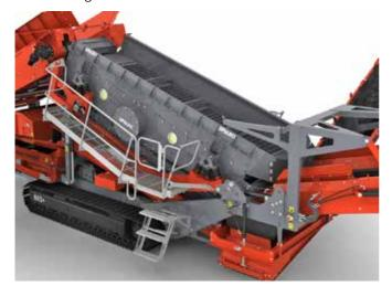
Thanks to their modular construction, the 3D screen segments with maximum open screen area can be quickly changed when necessary. The screen mats of the 3D Flip-Flow screen, are fastened without screws and have no edges that could cause difficulties.
