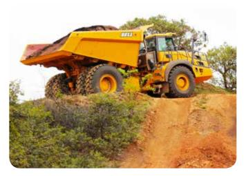
A key advantage of Bell Equipment's B60E over small rigid trucks is its all-wheel traction and retardation, which enables the truck to safety continue working in adverse weather conditions with no loss in production.
