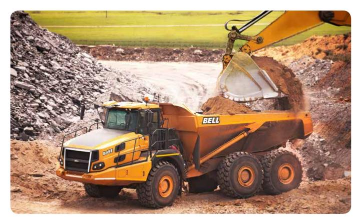
After three and a half years of development, and following the textbook introduction of its E-series Small Trucks in 2013, Bell Equipment will commence production of its E-series Large Trucks towards the end of 2016. Representing this range at Bauma 2016 was the B45E with a rated payload of 41 000kg and a bin volume of 25m<sup>3</sup>.
