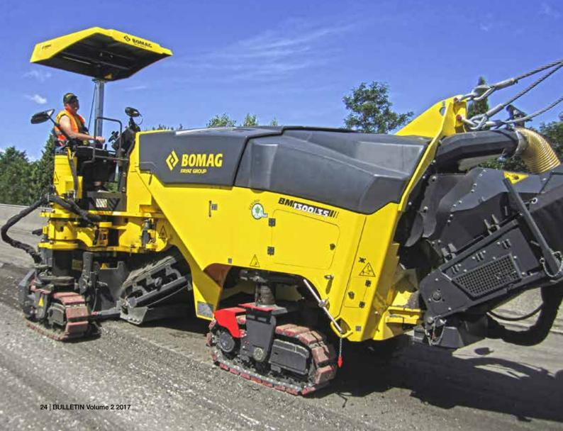
The range has a compact design which, together with their manoeuvrability, makes them an ideal choice for the removal of road and floor pavements under confined conditions and equally capable on arterial roads.
