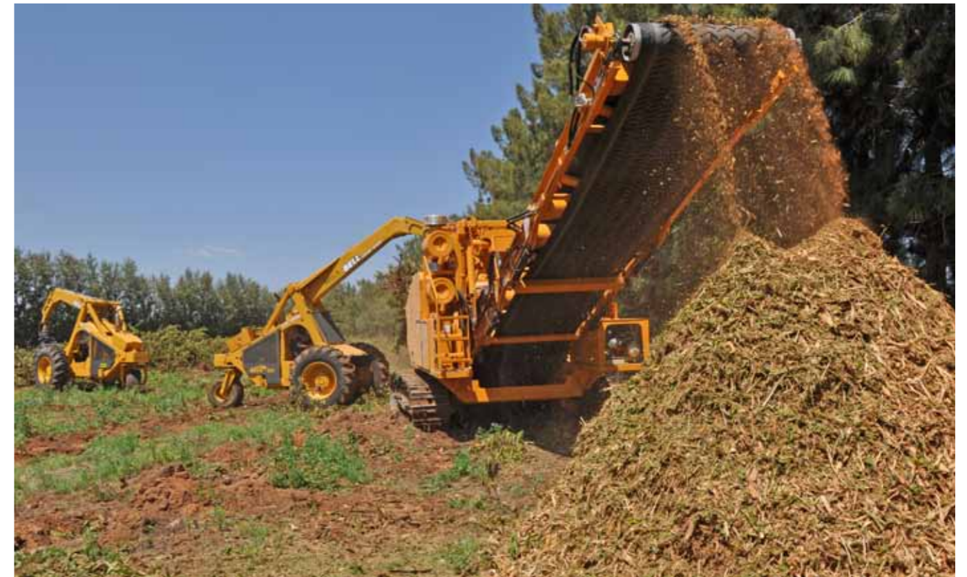
Whether it's removing windrows, or old fruit orchards, W.P. Chipper has a winning fleet of Bell 22A Loggers and wood-chippers to serve farmers in the Western Cape. The Bell Loggers are real workhorses responsible for moving felled trees and feeding them into the wood-chipper.
