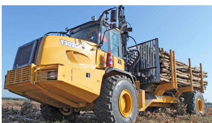
a ROPS/FOPS structure and provides superior operator comfort. "A sky roof optimises visibility when the crane is in operation while Lexan windows provide added safety. Likewise the cab guarding is ray orientated to limit dead zones and improve visibility," said Beningfield.
