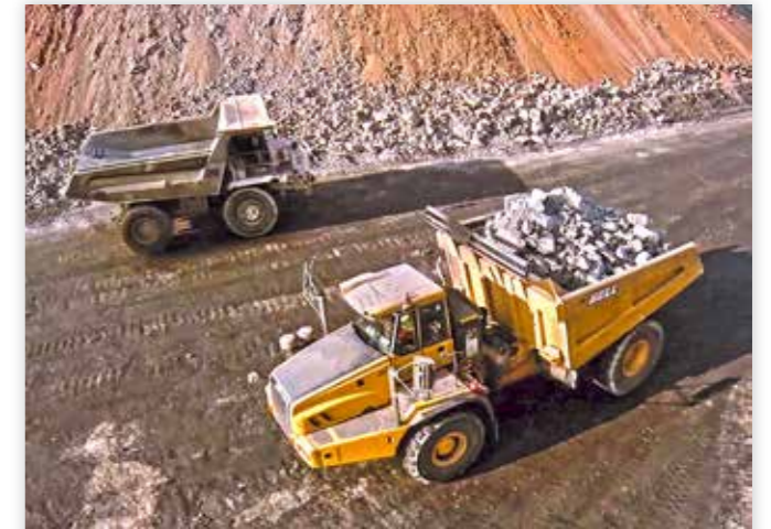
The completely new ADT concept, the B60D, has proved itself very successful in practice. Early in 2017 the EU/IV/Tier 4 final version of the B60E will be available.
