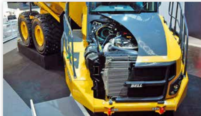
With this “sectional model” Bell Equipment presented the new Mercedes-Benz engines, which now feature on their smaller E-series B25E and B30E trucks.
