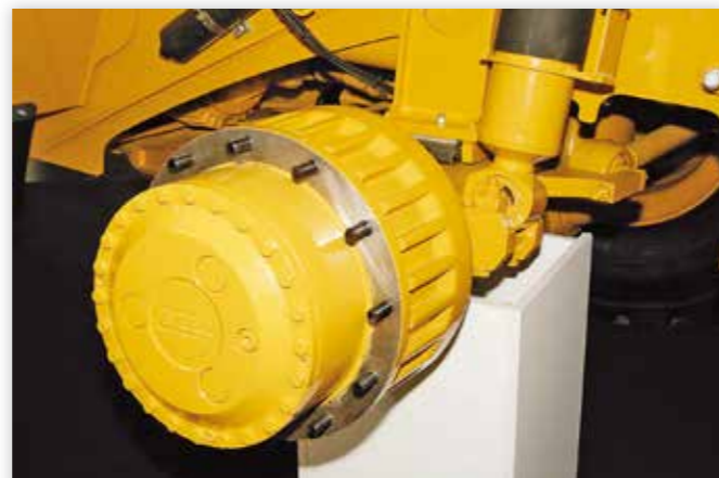
The optional active front suspension on the B25/30E with pressure accumulators (left) and active damper (right).
