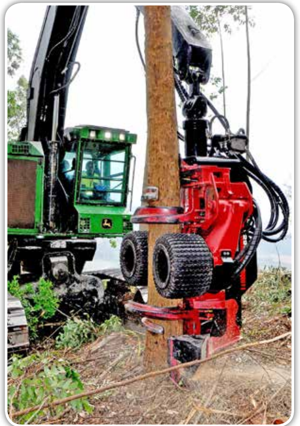
The H290 is a powerful, high-capacity head which features the highly efficient SuperCut 100 saw unit and can fell and process trees up to 760mm in diameter and debark and debranch to as thin as 50mm in diameter.
