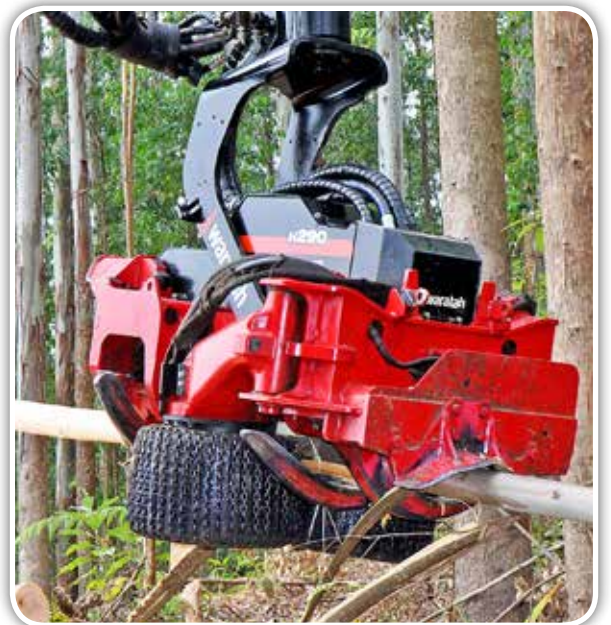
The use of special hydraulically driven rubber feed rollers on the Waratah H290 minimises mechanical damage to poles, as which is currently experienced in traditional mechanised pulp log debarking.
