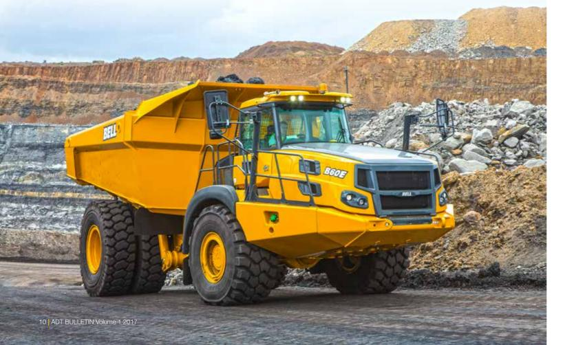
Safe Tip, downhill speed control and auto 4x4 traction control. Other standard features include auto grease systems, rearview camera, onboard diagnostics, and Bell's Fleetm@tic® telematics with full production data reporting.
