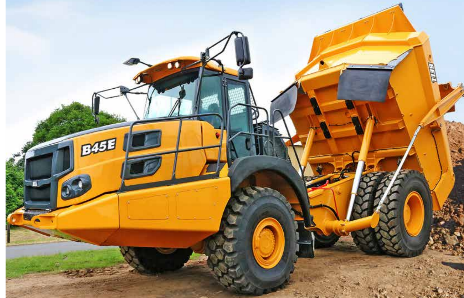
The 25m 3 rock bin of the Bell B45E 4x4 offers a low tipping height at crusher housings or in underground applications.
