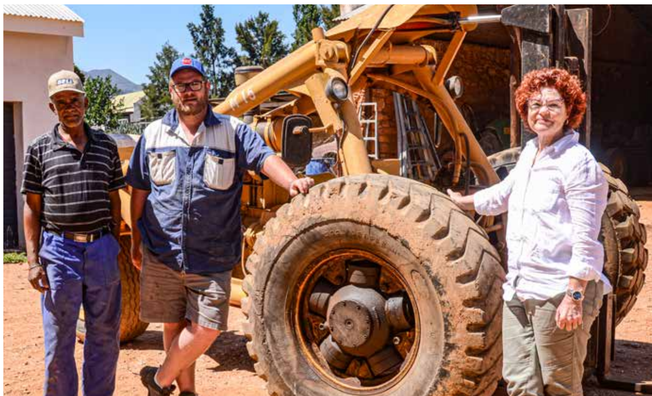
Forklift operator, Andrew America, Johann Reinecke and Bell Sales Representative, Fiona Johnson, with the Bell Forklift. Note the use of round tubing and the wheel motor visible on the outside of the wheel.
