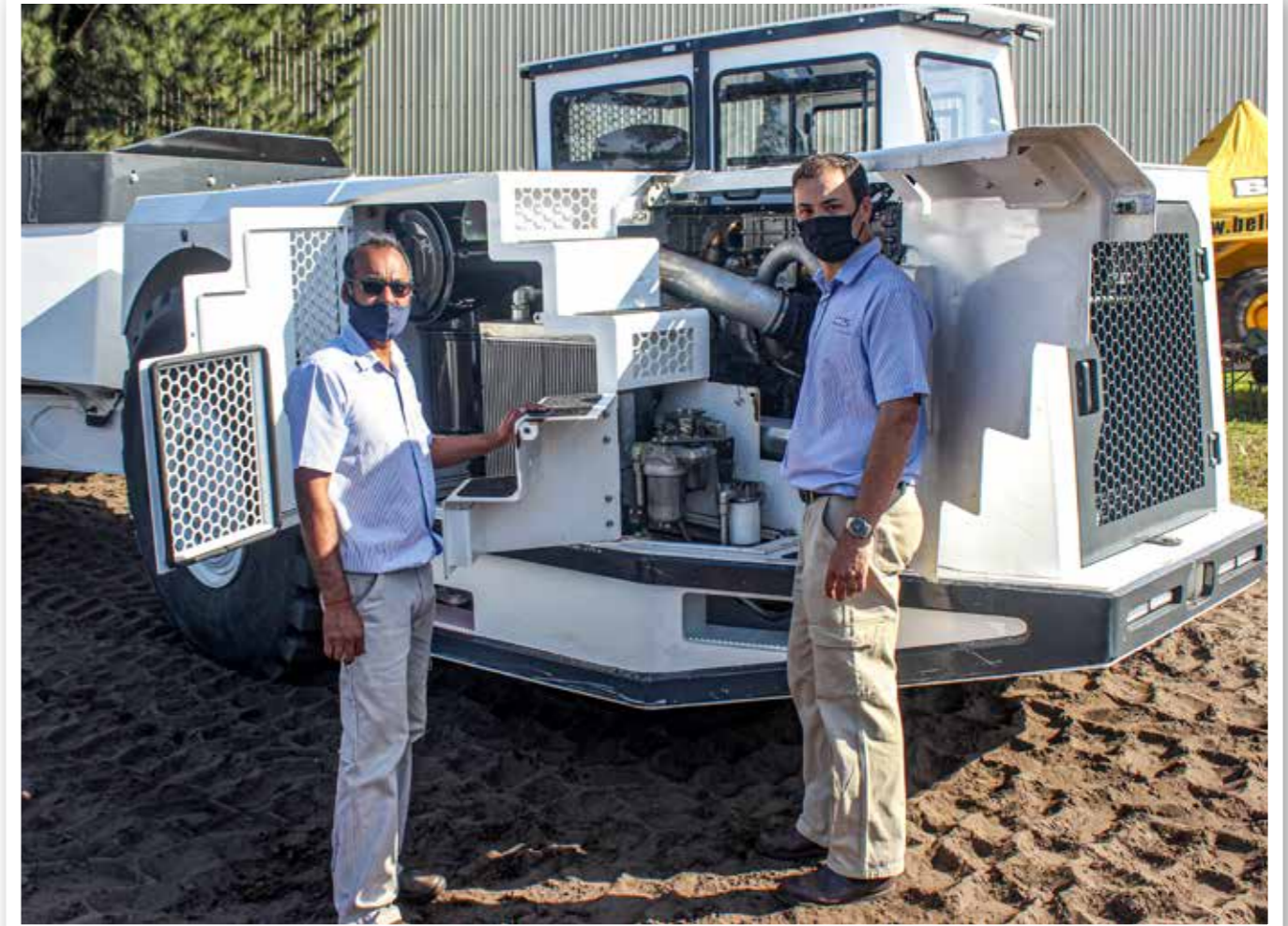
Bell Electrical Product Designer, Ashern Ramesar, and Product Designer, Shaun Tucker, demonstrate the easy ground level access for maintenance.
