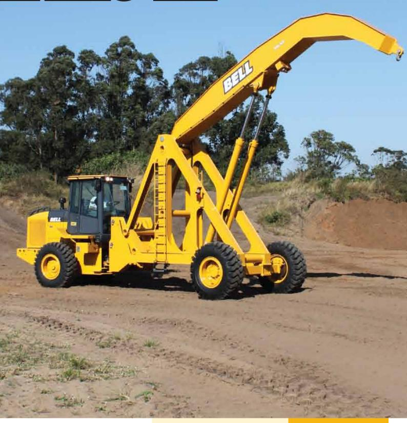
Net Peak Power : 95 kW Lift Capacity: 10 000 kg Operating Weight : 24 309 kg
