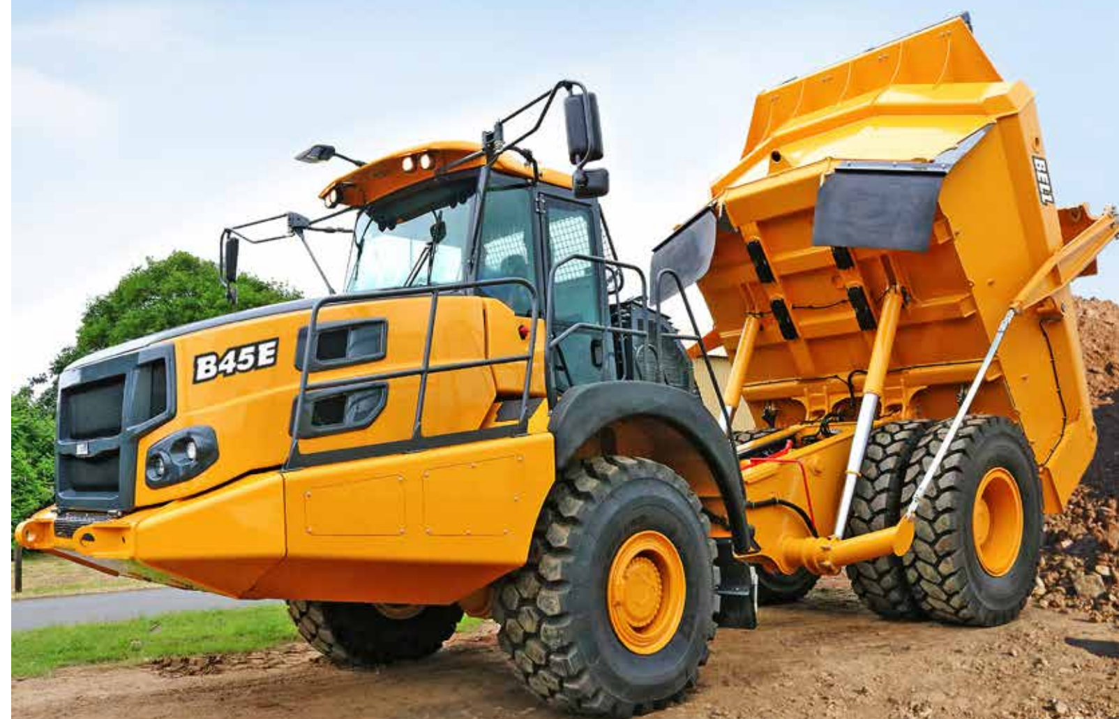
The 25m³ rock bin of the Bell B45E 4x4 offers a low tipping height at crusher housings or in underground applications.
