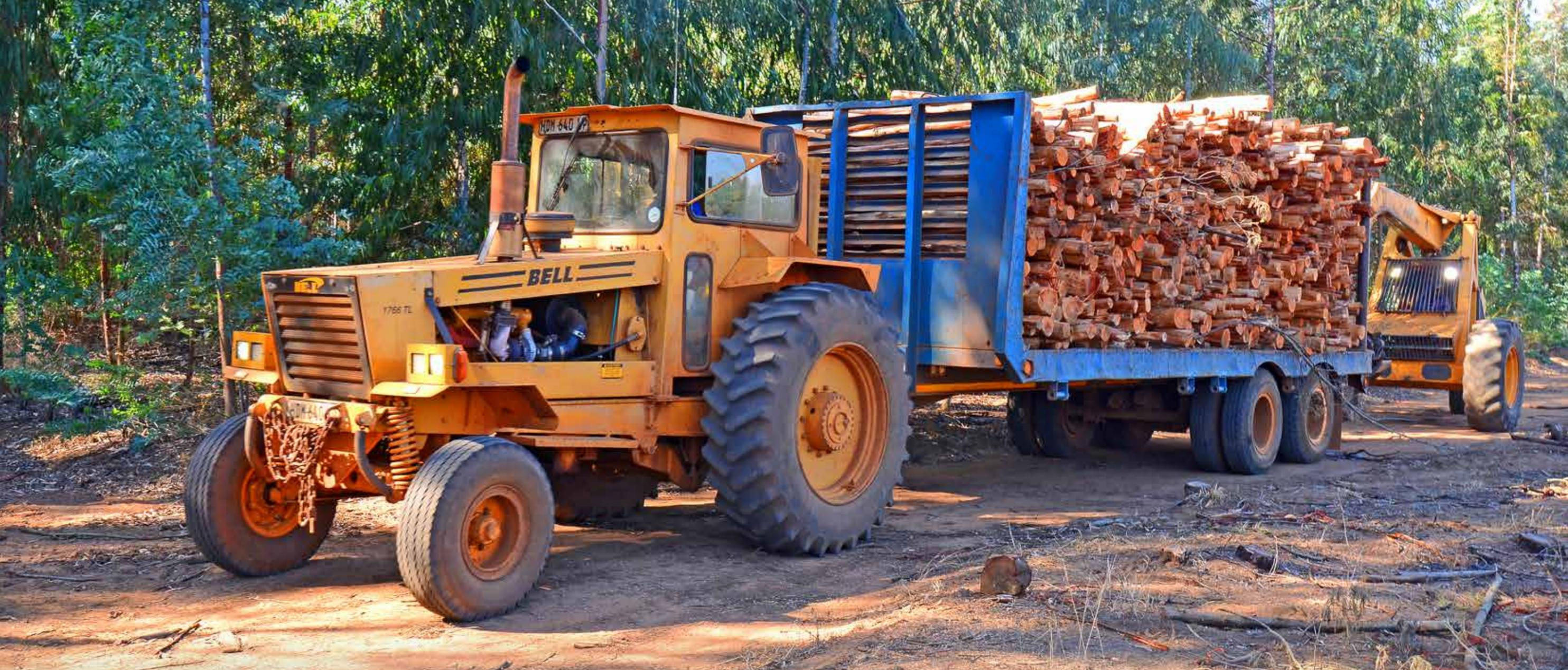
“We run five Bell 1766 Haulage Tractors, some of which we bought on the pre-owned market, and they are very hard to find, for good reason,” Ernst says. “Bell Equipment has perfected this machine as a haul tractor configuration especially when it comes to fuel consumption which is low at between 7 and 8 litres of diesel an hour, even when hauling 20 tons of timber.”
