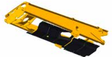
Underside belly plates
