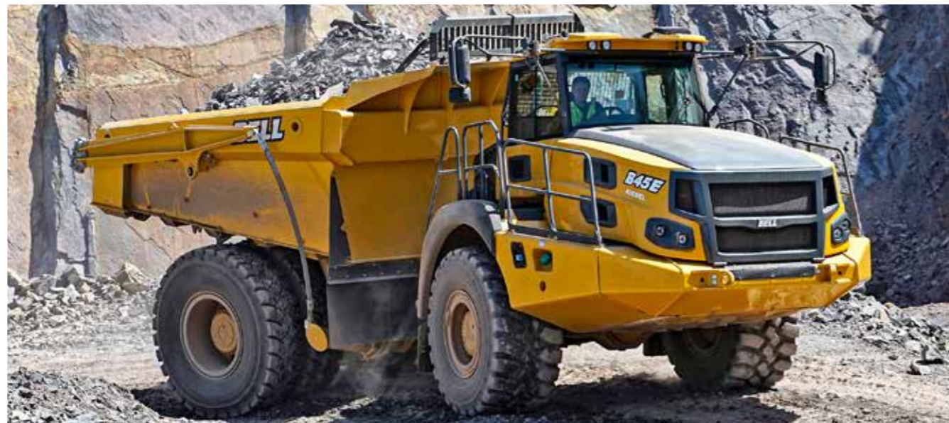
The 25m³ rock bin of the Bell B45E 4x4 offers a low tipping height at crusher housings or in underground applications.
