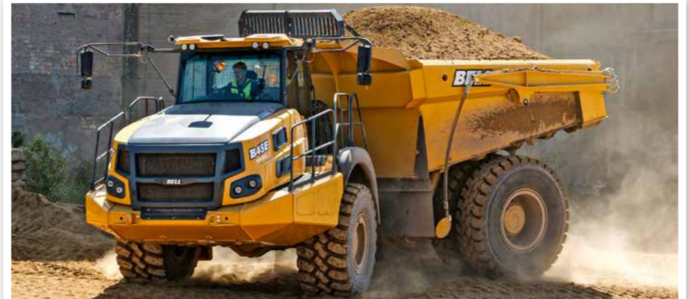
The B45E 4x4 has successfully brought the conceptual advantages of Bell Equipment's two-axle ADT to the 40-tonne payload class.
