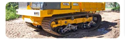
In addition, the walking beam geometry is biased, reducing the rear roller lift and track tension whilst traversing obstacles. The balanced system tracks the surface of the terrain better, providing chassis stability by not lifting the vehicle as high. This results in reduced ground pressure, lower track point-loading for longer track life, and improved operator comfort.
