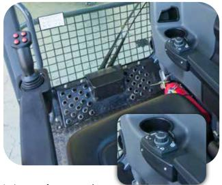
In terms of ergonomics, a single joystick control extends from the left-hand side armrest from which electric over hydraulic control of all forward, left, right and backward machine movements are controlled. Additional functions, such as raising and lowering the dump bed, cruise control and sounding the horn, are assigned to buttons on the joystick. For safety, all joystick functions require that the pilot switch be pressed for the functions to work.
