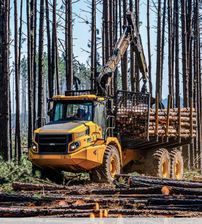
Designed with safety and ease of operation in mind; safety critical operations, such as the park brake and crane functions, are automatically applied or limited in unsafe conditions. Automatic Traction Control (ATC) is achieved through the automatic application of the Inter-axle Differential Lock (IDL) while driving.
