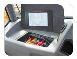
An in-cab load center simplifies fuse replacement. Fewer relays, connectors and harnesses mean higher reliability.
