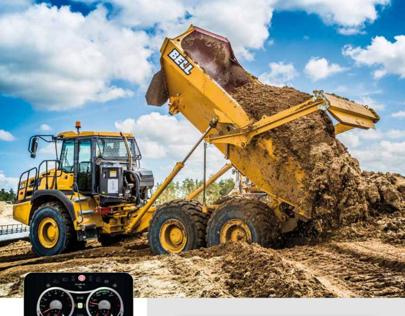
The incorporation of a pitch and roll sensor in the vehicle prevents bin operation if the truck is in an unsafe position.
