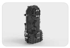
The transfer case inter-axle differential delivers equal torque to each axle when traction is favorable. When conditions deteriorate, the diff-lock automatically engages to deliver torque to the tires that can best use it.
