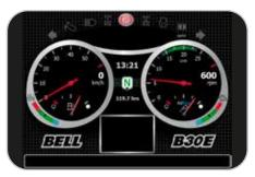
A user friendly 10" color monitor offers vital operating information, safety warnings, detailed diagnostic readings and dump body function settings.
