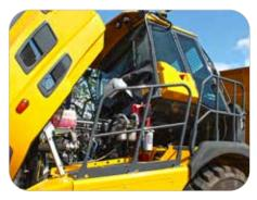
The cab can be tilted in minutes without special tools, for convenient service access to drivetrain components.
