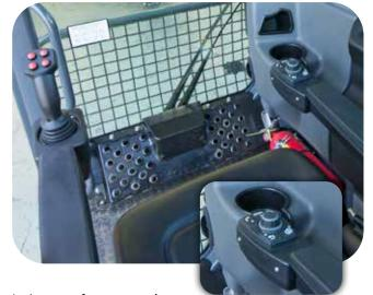
In terms of ergonomics, a single joystick control extends from the lefthand side armrest from which electric over hydraulic control of all forward, left, right and backward machine movements are controlled. Additional functions, such as raising and lowering the dump bed, cruise control and sounding the horn, are assigned to buttons on the joystick. For safety, all joystick functions require that the pilot switch be pressed for the functions to work.
