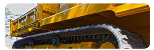
In addition, the walking beam geometry is biased, reducing the rear roller lift and track tension whilst traversing obstacles. The balanced system tracks the surface of the terrain better, providing chassis stability by not lifting the vehicle as high. This results in reduced ground pressure, lower track point-loading for longer track life, and improved operator comfort.
