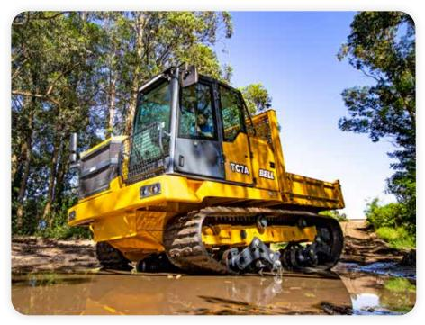
• Bell manufactured components – Design and manufacture philosophies that have been adopted from our decades of ADT successes have been instilled into the Tracked Carrier. The steel structures, including the cab, structures and track suspension system, are run through independently developed and globally recognized processes such as Finite Element Analysis (FEA) testing to ensure maximum durability.
