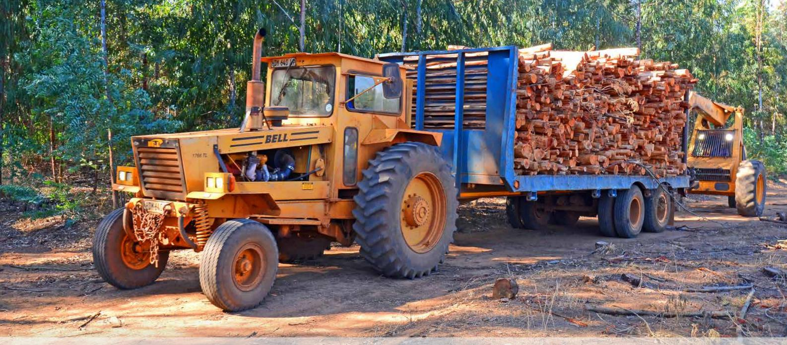
"We run five Bell 1766 Haulage Tractors, some of which we bought on the pre-owned market, and they are very hard to find, for good reason," Ernst says. "Bell Equipment has perfected this machine as a haul tractor configuration especially when it comes to fuel consumption which is low at between 7 and 8 litres of diesel an hour, even when hauling 20 tons of timber."
