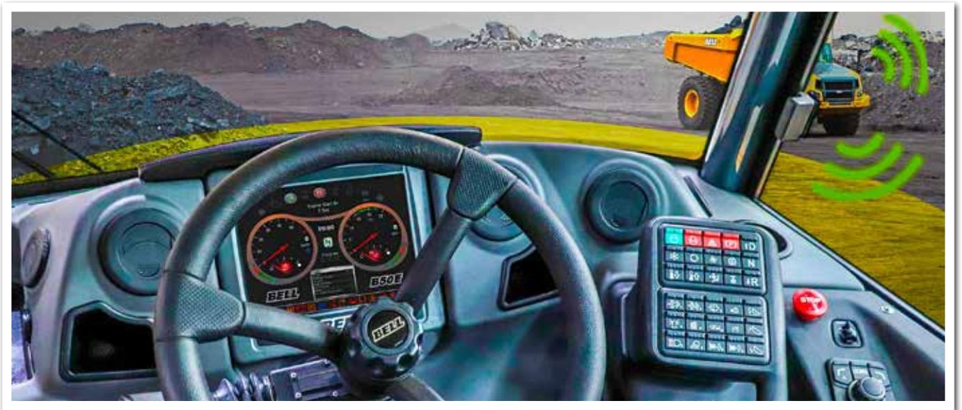
In terms of the regulations, diesel-powered, trackless mobile machines must be able to automatically detect the presence of pedestrians and other diesel-powered, trackless mobile machines in the vicinity, and provide an effective warning. Where no action is taken to prevent a potential collision, the machine must be able to “fail to safe” without human intervention by means of a system that has the means to retard the machine to a safe speed whereafter the brakes are autonomically applied.
