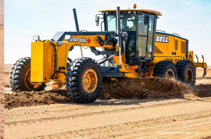
This is complemented with a reverse camera and mirror. Designed to operate in high ambient and dusty environments, the cab is equipped with a powerful air conditioner and optional air cleaner to ensure an ergonomic and clean environment for the operator. "Maintenance has been incorporated into every aspect of the design by leveraging the insights of a number of plant managers and directors as well as analysing our extensive historical maintenance and repair logs," continues Warren.
