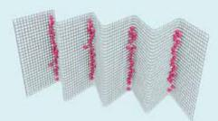
•30-mesh means that there are 30 holes formed by horizontal and vertical wires in every square inch of filter.
