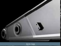
Thickness of steel plate has been increased.
