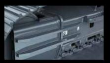
Reinforced Guide Frame Reinforced guide frame prevents deformation caused by impact or encroaching of loose stones.
