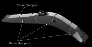
The XD boom features stronger plates compared to the HD booms of standard machines, which increases longevity even under the toughest working conditions. **Big cross-section boom**
