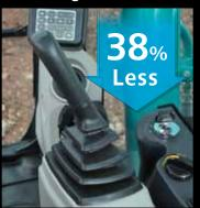
It takes 38% less effort to work the operation lever, which reduces fatigue over long working hours or continued operations.
