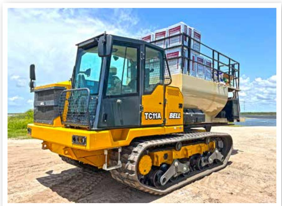
**The versatile Bell Tracked Carrier can be used to carry attachments such as hydroseeders.**
