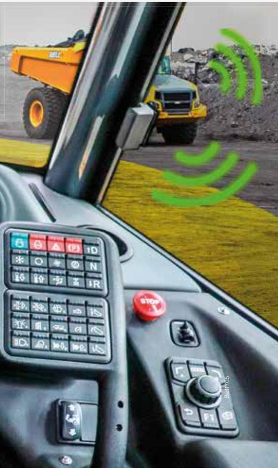
\* Proximity Detection System / Collision Avoidance System
