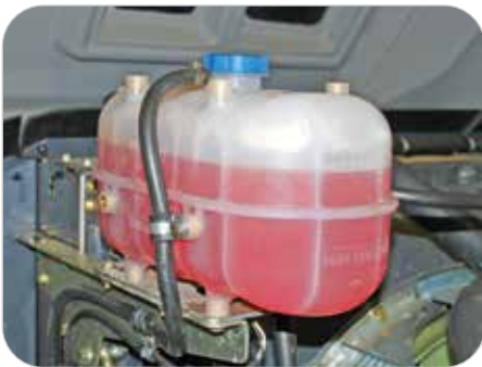
See-through fluid reservoirs and sight gauges let you check fluid levels at a glance.
