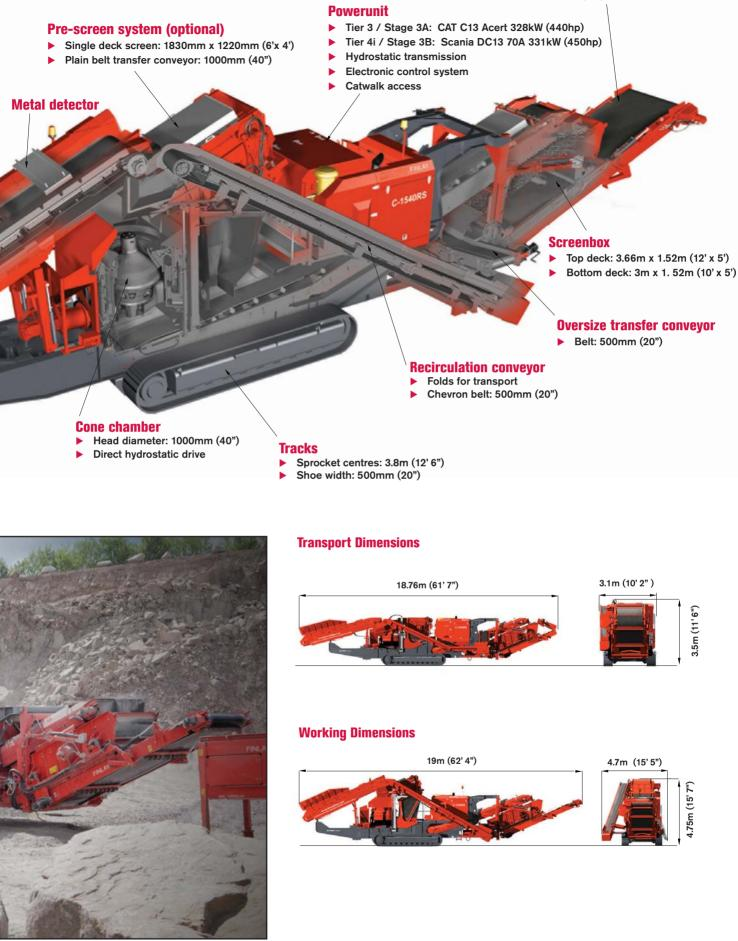
Machine Weight: 43,800kg (96,563lbs) Without options 45,600kg (100,531lbs) With optional pre-screen 49,000kg (108,027lbs) With optional pre-screen, mid-grade transfer & mid-grade stockpiling conveyor
