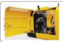
Remote-mounted engine oil filter to allow easy access.
