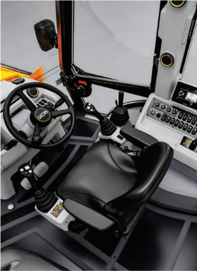
Inside the JCB 3CX Pro: all cabs are ROPS/FOPS certified with improved cab sealing.
