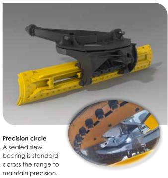
It delivers consistent mouldboard accuracy due to minimal wear and requires less maintenance compared to open gear designs. Furthermore, adjustable mouldboard inserts can be adjusted in five minutes and are designed to maximise the life of the wear inserts.
