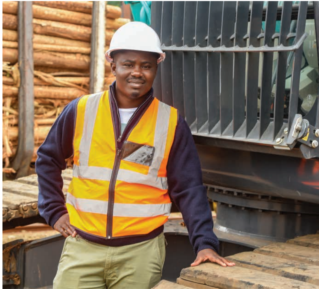
Simphiwe Magubane, owner of Goobs Forestry (Pty) Ltd, showing the rubber pads on the tracks of the Kobelco SK220XD-10 Excavator.
