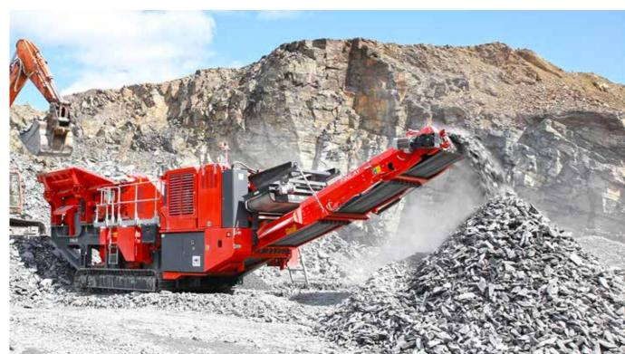
The plant incorporates the robust and renowned JW42 high performance electrically driven single toggle jaw chamber and a heavy duty VGF feeder to give optimum production in quarrying, mining, demolition and recycling applications. Additional benefits include rapid set up time, ease of maintenance, high reduction ratio, high output capacity and advanced electronic control system.
